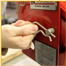
Clevis style pins for quick release, boom adjustments, and fold down for storage.
