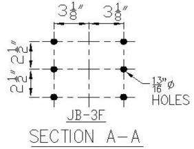
NOTE; JIB ASSEMBLY BOLTS & COLUMN CONNECTION BOLTS. TO BE ASTM-A-325 PER A-H CO. RECOMMENDATION.
