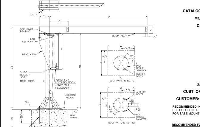
J904B BASE MOUNTED JIB CRANE GENERAL ARRANGEMENT
