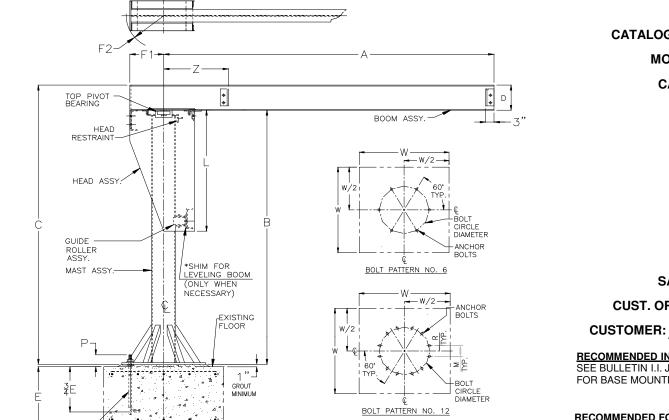
J904B BASE MOUNTED JIB CRANE GENERAL ARRANGEMENT
