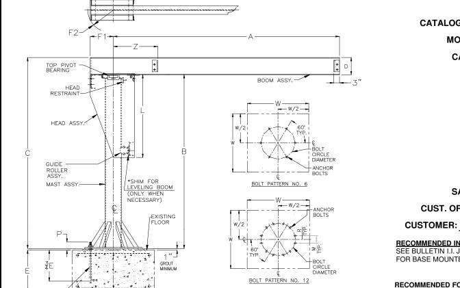
J904B BASE MOUNTED JIB CRANE GENERAL ARRANGEMENT
