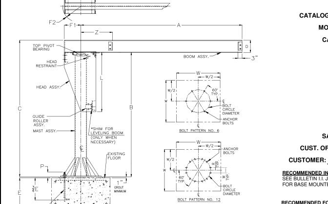
J904B BASE MOUNTED JIB CRANE GENERAL ARRANGEMENT
