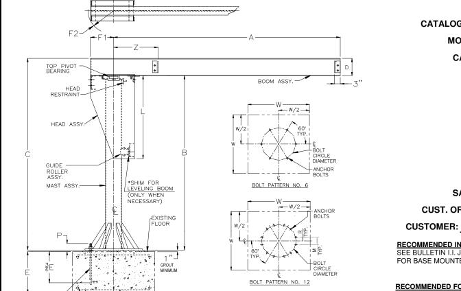
J904B BASE MOUNTED JIB CRANE GENERAL ARRANGEMENT
