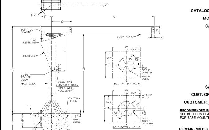
J904B BASE MOUNTED JIB CRANE GENERAL ARRANGEMENT
