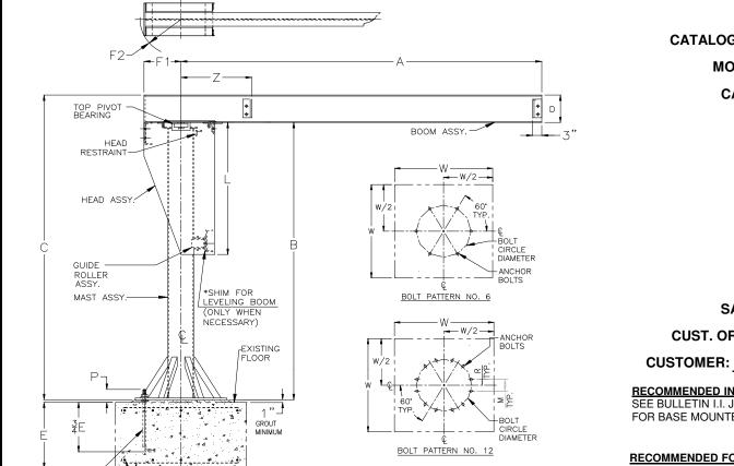
J904B BASE MOUNTED JIB CRANE GENERAL ARRANGEMENT
