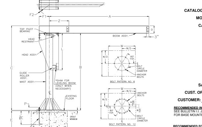
J904B BASE MOUNTED JIB CRANE GENERAL ARRANGEMENT
