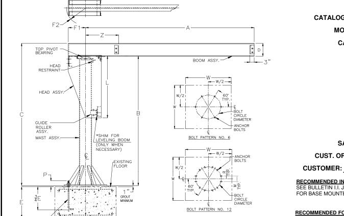
J904B BASE MOUNTED JIB CRANE GENERAL ARRANGEMENT
