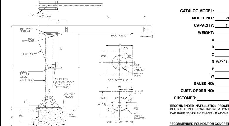
J904B BASE MOUNTED JIB CRANE GENERAL ARRANGEMENT NOTE: 1. BASE PLATE O.D. 6" LARGER THAN BOLT CIRCLE. \*2. MODEL NO. 300 (HEAVY), 360 & 420 HAS SHIMS ON TOP OF HEAD ASSY, UNDER BOOM.
