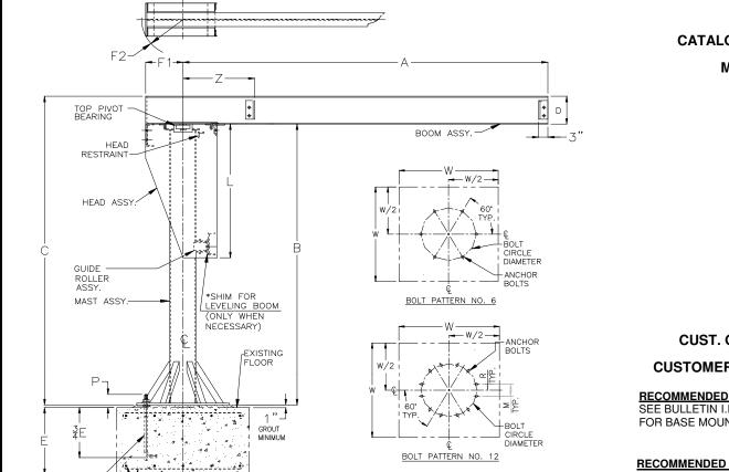
J904B BASE MOUNTED JIB CRANE GENERAL ARRANGEMENT
