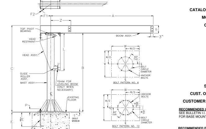
J904B BASE MOUNTED JIB CRANE GENERAL ARRANGEMENT
