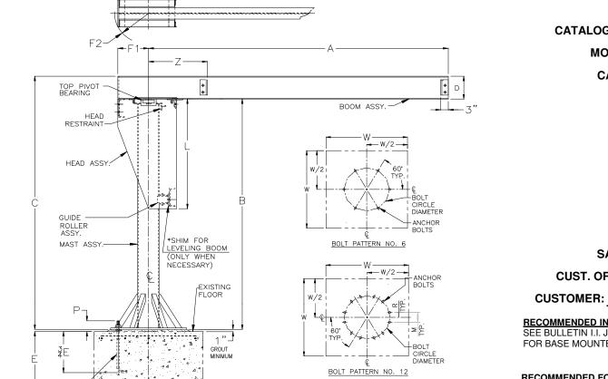
J904B BASE MOUNTED JIB CRANE GENERAL ARRANGEMENT
