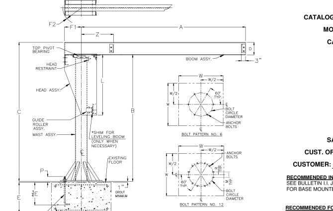
J904B BASE MOUNTED JIB CRANE GENERAL ARRANGEMENT
