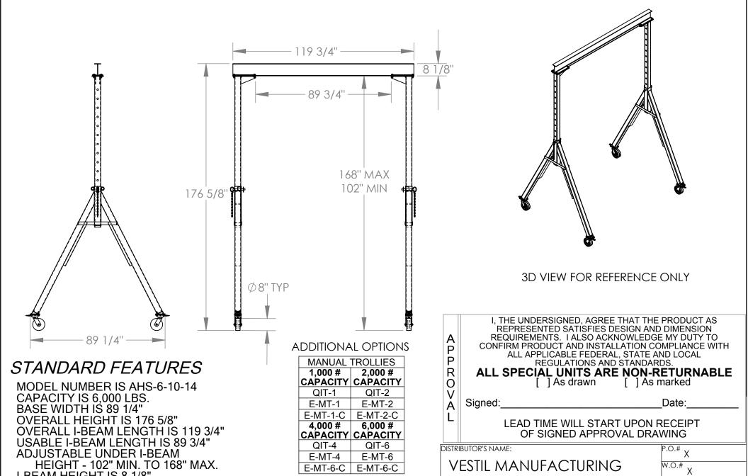
HEIGHT - 102" MIN. TO 168" MAX. I-BEAM HEIGHT IS 8 1/8" (4) Ø8" SWIVEL CASTERS WITH FOUR LOCKING POSITIONS
