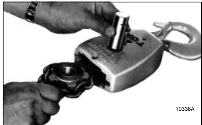
Figure 7-29. Removing Coil Chain and Sprocket on 2 thru 5 Ton Lower Block Assembly (Link Chain Model)
