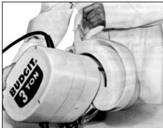
Figure 7-3. Removing 3 Ton Hanger Bracket from Hoist Frame
